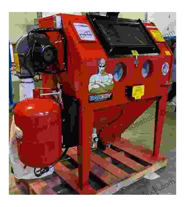
Media blasting equipment includes a blast pot, air compressor, and nozzle. The blast pot holds the abrasive material, which is then propelled through the nozzle by a stream of compressed air. The nozzle can be adjusted to control the size and shape of the spray pattern.
